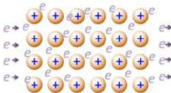
Fig.7.2: Schematic representation of electrical conduction by metals in terms of electron sea model
