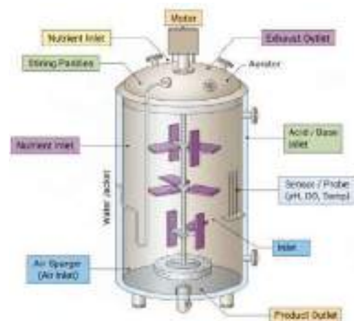
Figure 5: Parts of a fermenter
